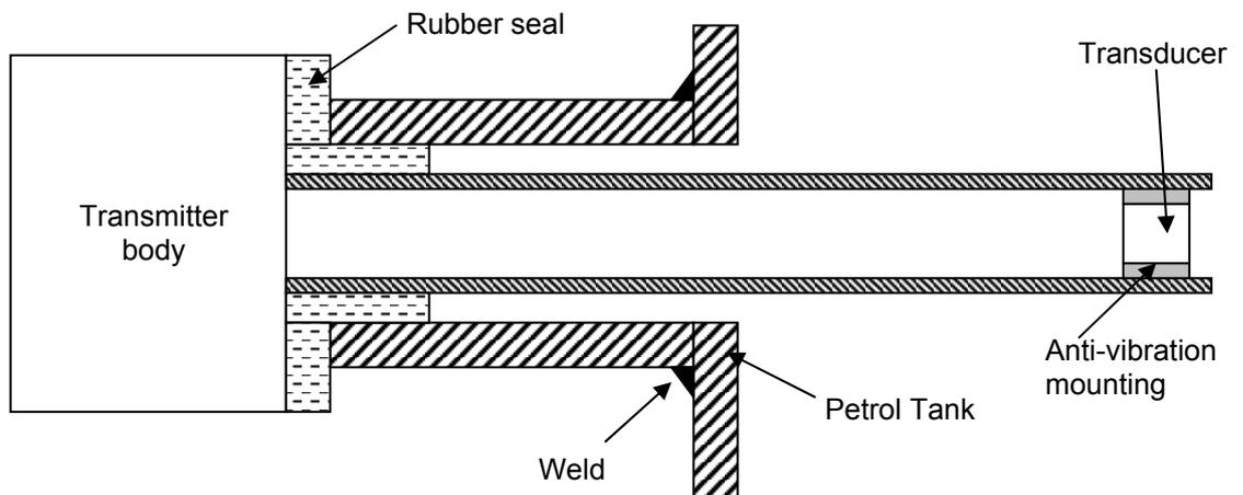
The test process is to firstly close the inlet/outlet pipes and fit the ultrasound transmitter.
