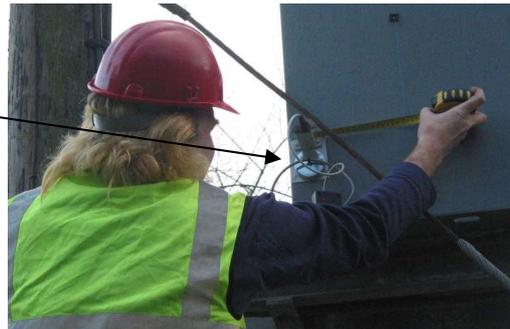
A consistent signal input was supplied by means of a fixed pendulum with a measured swing. This would ensure that the same force of impact was used in both the controlled and test applications for both units. In order to maximise any influence of noise on the signal a very low impact force was used and the DrX units set to high sensitivity.
