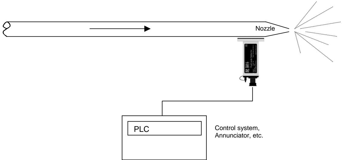
Again the logic is very simple since failure of any signal suggests either no process liquid or a blocked nozzle.
