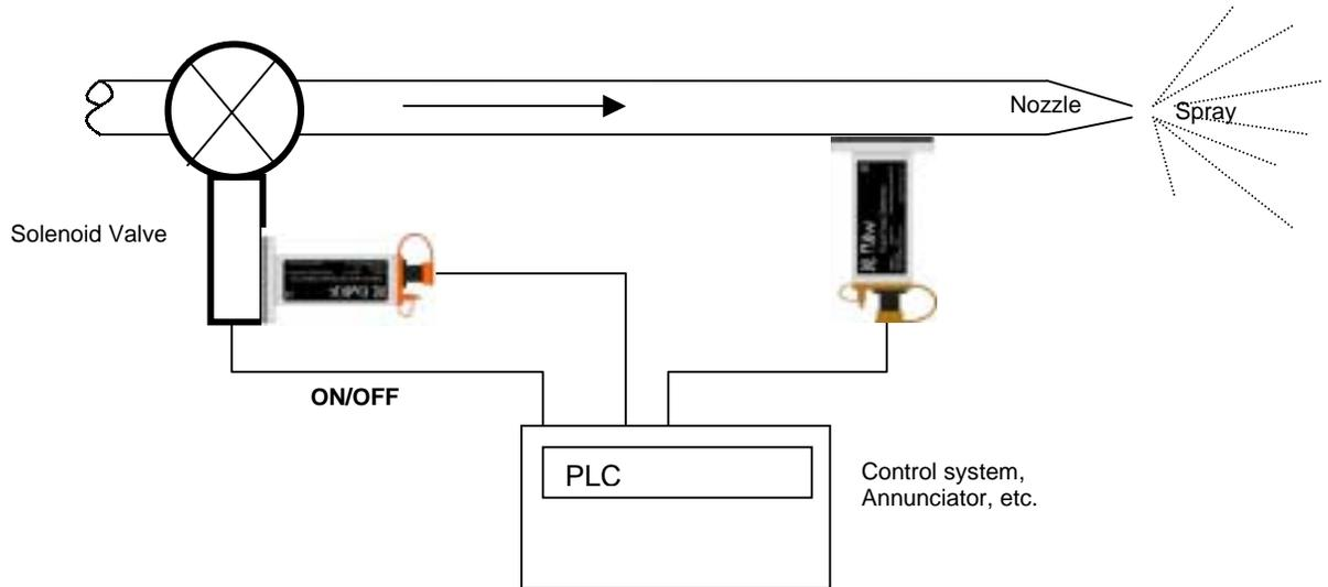
Fitting a DrKnock, mechanical noise detector, to the solenoid valve will indicate to any simple control system that the solenoid has moved, and consequently flow should start or stop within a given time. The result of this valve movement can be confirmed downstream by means of a DrFlow, liquid flow detector.
